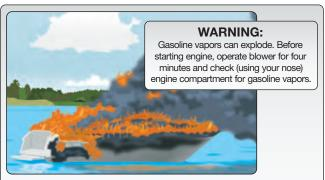
Vessels built after July 31, 1980, that contain power exhaust blowers in gasoline engine compartments must have the above warning sticker placed near the instrument panel.
